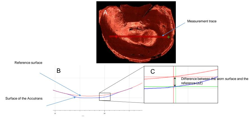
Measurement of the wear scar depth on the meniscus using an Alicona IF G5 optical microscope from Accutrans replicas:
