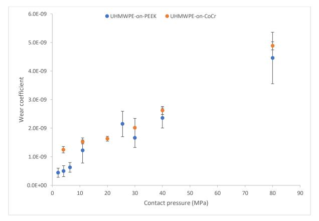
Mean wear coefficient ± 95% confidence limits of UHMWPE pins articulating against PEEK-OPTIMA<sup>™</sup> plates under contact pressures from 2.1 to 80 MPa, minimum n=5. Data compared to the mean wear factor ± 95% confidence limits of moderately cross-linked UHMWPE-on-CoCr (cobalt chrome) of similar initial surface topography from Abdelgaied et al<sup>1</sup>.
